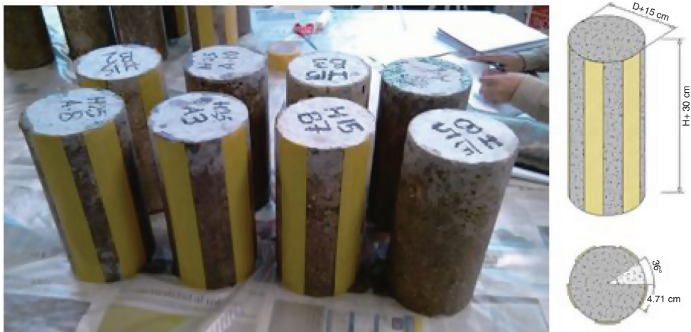
FIGURE 1. Photograph and diagram illustrating the 50% CFRP-reinforced specimens.
