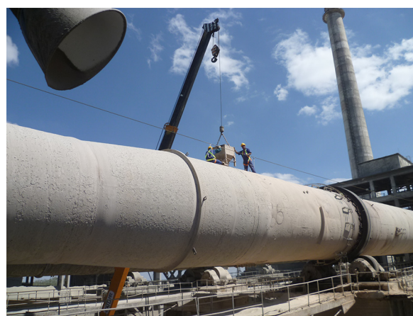
FIGURE 2. Direct feeding of the clay to the rotary kiln.
