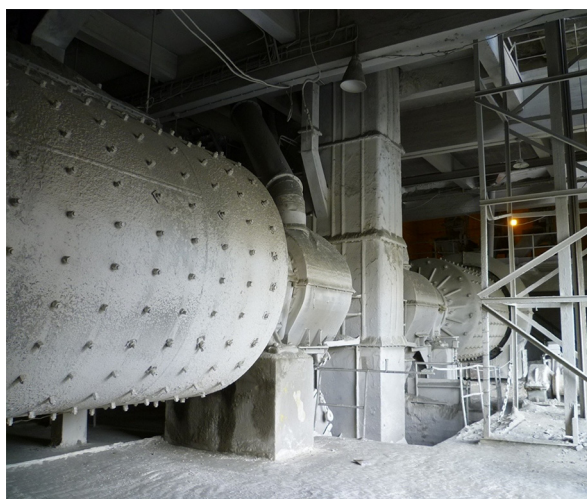
FIGURE 5. Industrial ball mill used to produce, through co-grinding; the low carbon cement.
