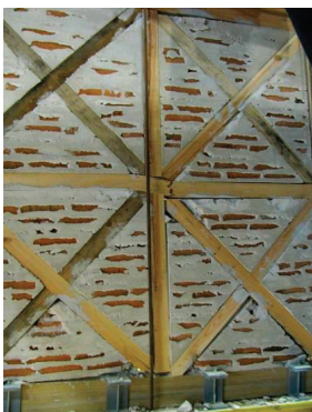
FIGURE 6. Failure mode of masonry walls MW1 and MW2.
