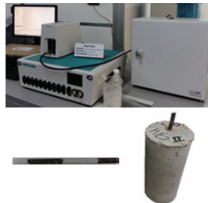
FIGURE 2. Setup for the electrochemical measurements of reinforced concretes exposed to carbonation.
