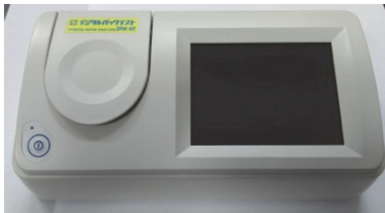
Figure 1: Digital pack test meter was used for the evaluation of inorganic nitrogen.
