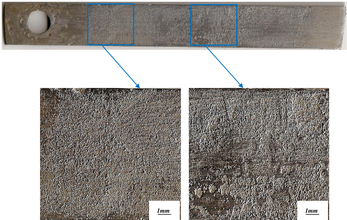
Fig.5.32 Pitting, coupon A10. CR (1,1683mpy).1200ppp.
