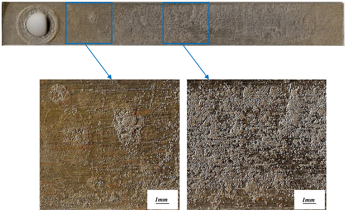
Fig.5.33 Pitting, coupon A15.CR (1,3923mpy) 1200ppp.
