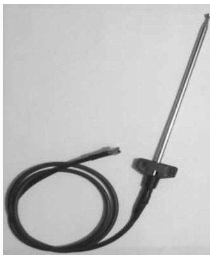
Figura 5-2: Antena dipolo simple.
