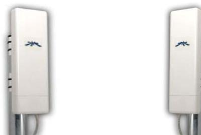
Figura: V.39: Antenas Ubiquiti Nanostation
