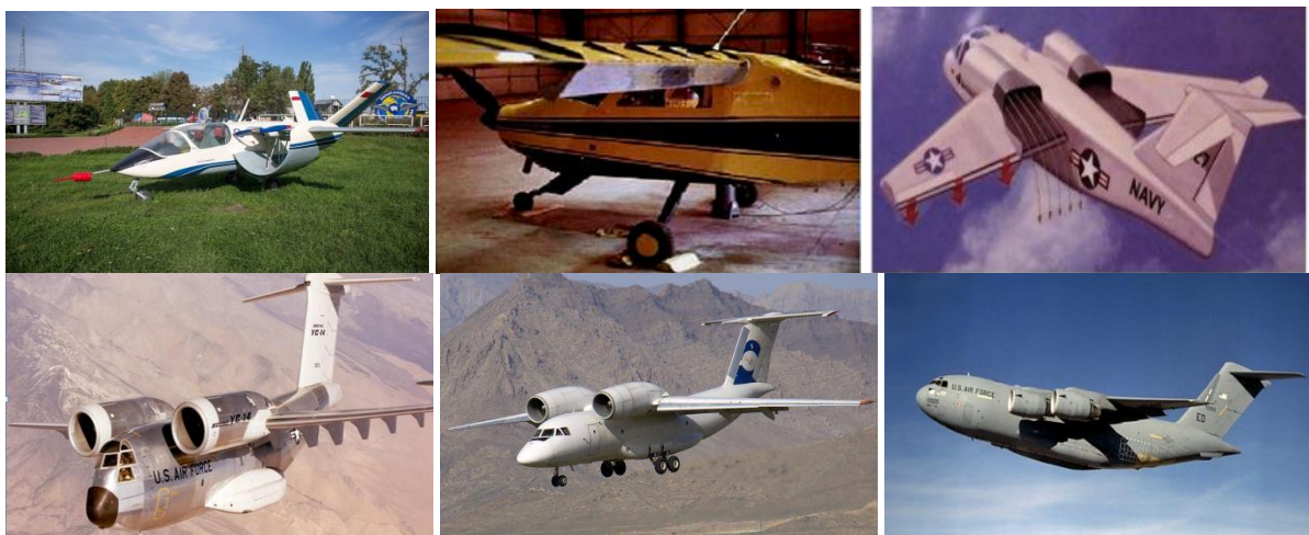
Figure 11: Coandă Effect implemented on aircraft a) Antonov Izdeliye 181 b)WVU Flight Demonstrator c) The Navy A-6/CCW demonstrator aircraft d) Boeing's YC-14 (1976) (AMST) e) The Antonov An-72, and f) The Boeing C-17 Globemaster III
