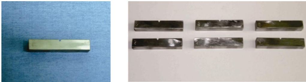
Fig. 6. Physical appearance of the impact toughness test samples.
