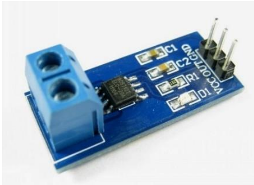
Figure 3. Hall effect-based linear current sensor ACS712
