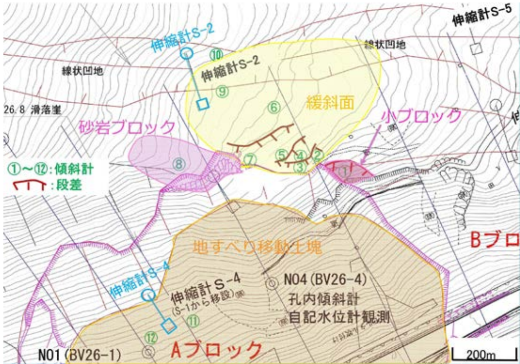
図8 計測装置の配置と周辺の地形 Fig. 8 Arrangement of monitoring devices and the topography around the monitored area.
