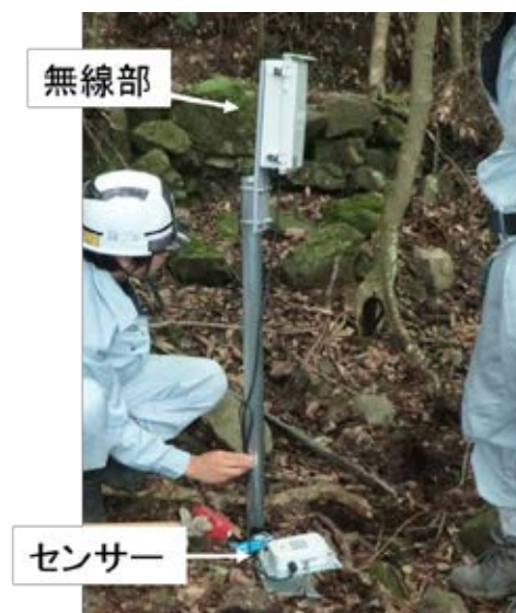
写真4 ばらまき型傾斜計(株オサシ・テクノス) Photo 4 MEMS tilt meter used for monitoring.
