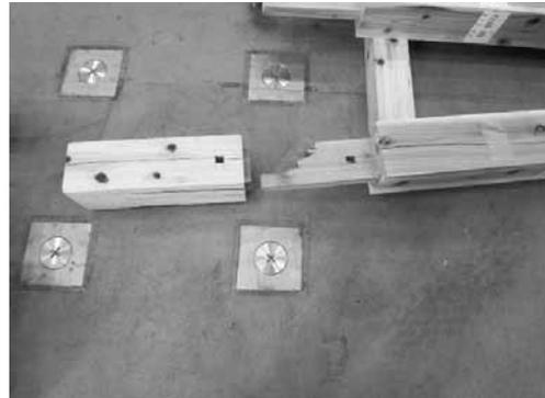
b) Breakage of Column-base X11-Y1 below horizontal tie
