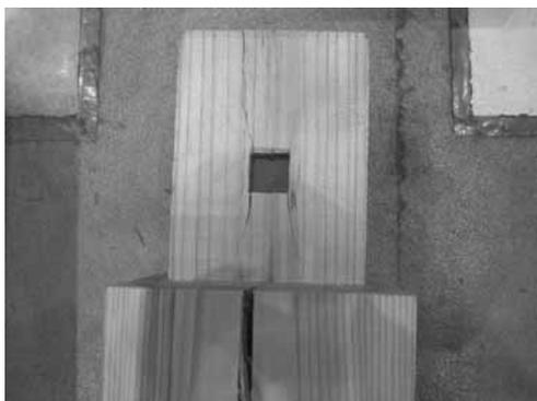
c) Cracks in Column-top X13-Y3 tenon
