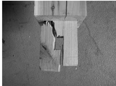
b) Breakage of Column-base X7-Y5 tenon
