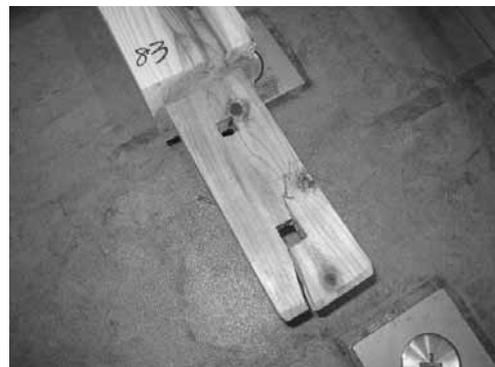
b) Breakage of Column-base X11-Y5 tenon below horizontal tie
