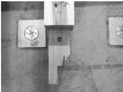
a) Breakage of Column-base X7-Y1 tenon
