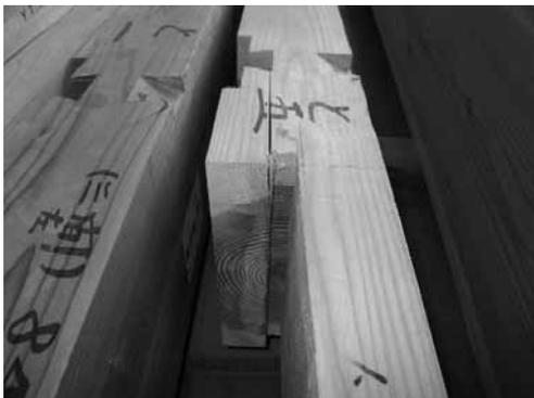
c) Splits in Horizontal Member X3-Y7 due to dislodged oblique scarf joint.
