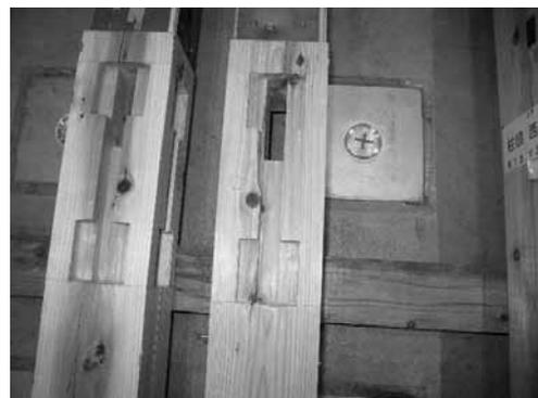
d) Crushing outward of Column-top X13-Y1 spline mortise
