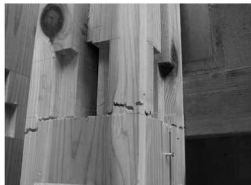
d) Breakage of Column-top X5-Y4 below structural lintel X13Y7.
