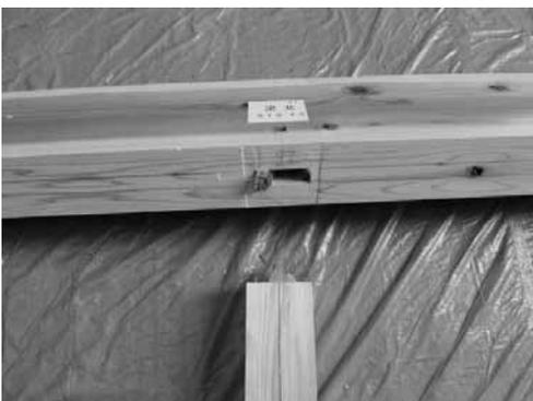
c) Breakage of Column-top X5-Y5 below horizontal member
