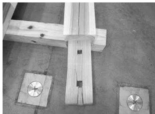
d) Breaking-off of Column X11-Y5 tenon-end
