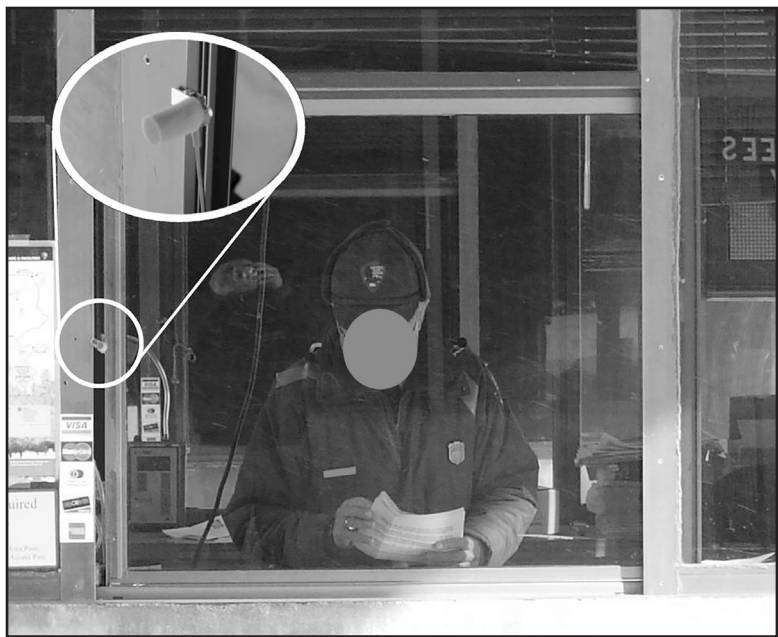
Figure 4. Microphone placement on the window frame of a kiosk during area monitoring at the West Entrance to YNP.
