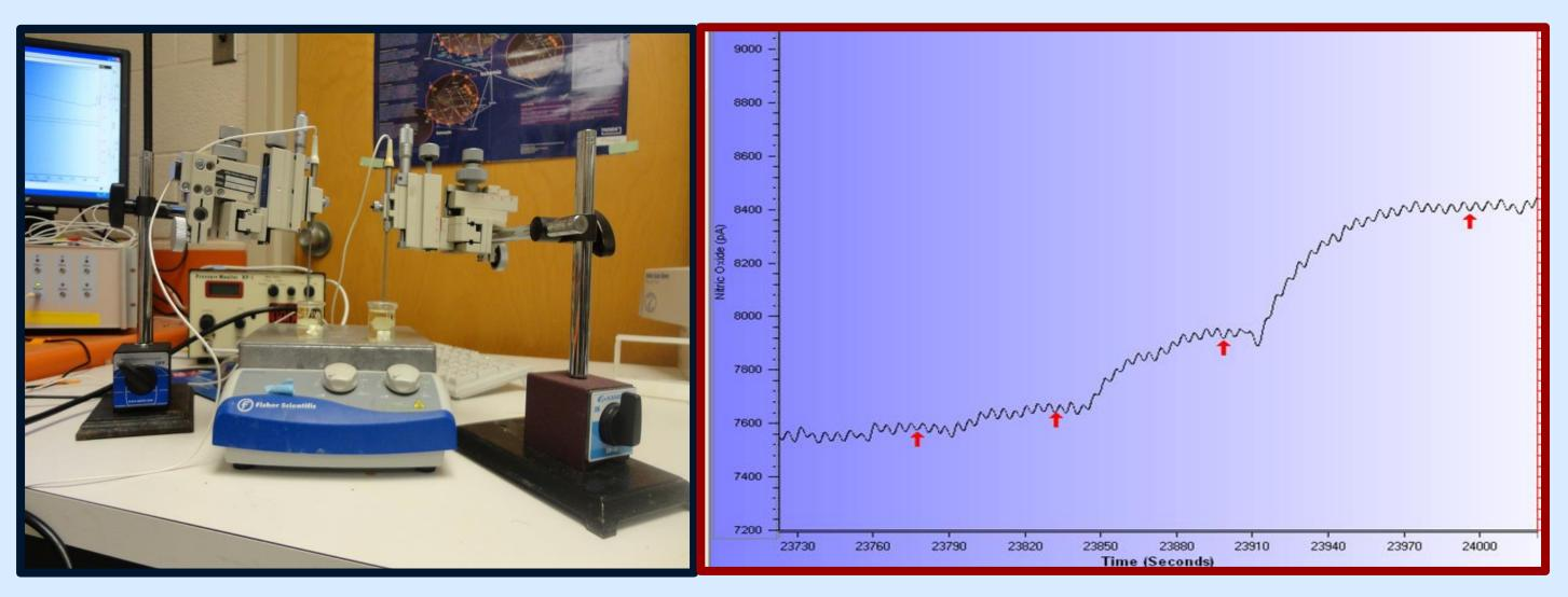
**Figure 3.** Illustration of NO electrode calibration setup (left), calibration curve (top right) and HUVEC NO measurement in 6-well plates (bottom). The NO electrode was calibrated based on the following reaction:  $2KNO_2 + 2KI + 2H_2SO_4 \rightarrow 2NO + I + 2H_2O + 2K_2SO_4$  (e.g. y = 0.9346x + 3.4828; R<sup>2</sup> = 0.997) that corresponded to a 25 nM to 200 nM range (right). Dose responses are indicated by red arrows.
