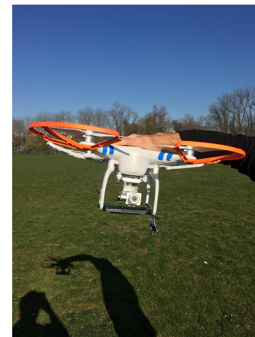
Figure 2. Our fully equipped DJI Phantom 2 Vision UAV, with the i-Phone 5 AliveCor ECG software mantled to the underside.
