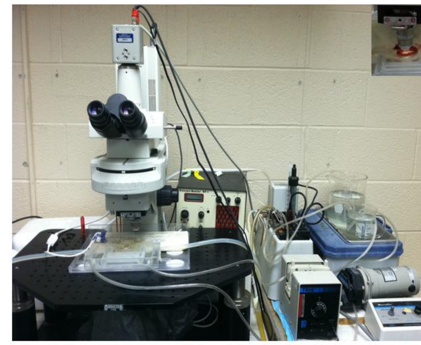
Figure 4. Experimental setup for intravital microscopy. Inserted picture in upper right: exteriorized loop of mesenteric tissue undergoing superfusion of test solution.
