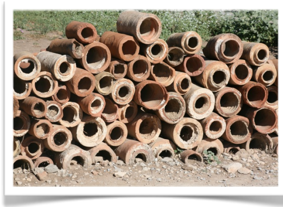
Figure 15. Terracotta pipes, found in the Agora, which show clear signs of sedimentation.
