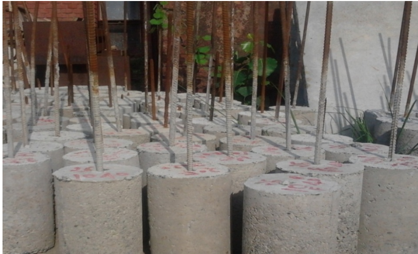
Figure 3: Cylindrical specimens after pull-out tests.
