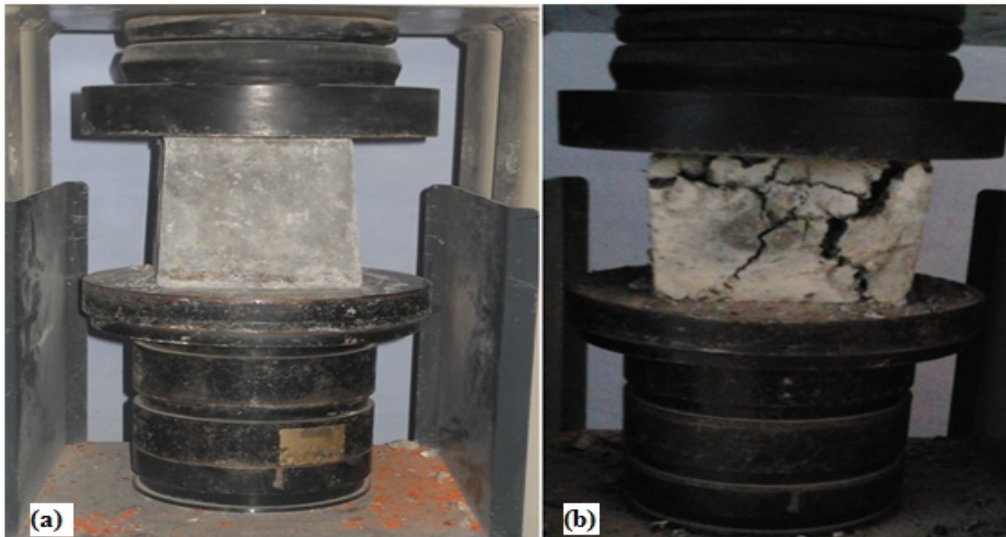
Figure 2: Cube specimen under compression testing before (a) failure (b) after failure.
