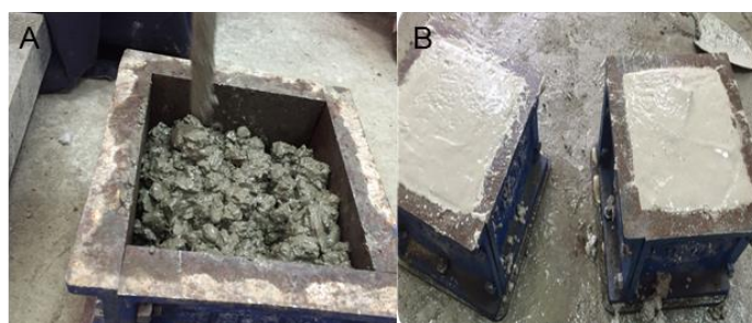
Figure 1 (A&B). Casting and Levelling of Concrete Samples.
