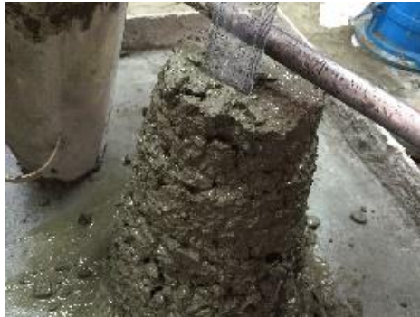
Figure 6. Slump test result for normal mix.
