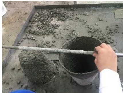
Figure 9. Slump test result for 1% Micro-Silica, 0.8% CF 615.
