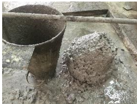
Figure 8. Slump test result for 1% nano-silica, 0.8% CF 615.
