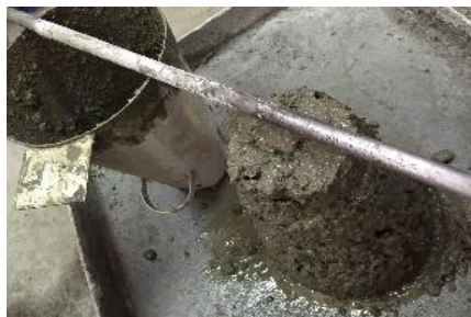
Figure 10. Slump test result for 1% Pozzolan, 0.8% CF 615.
