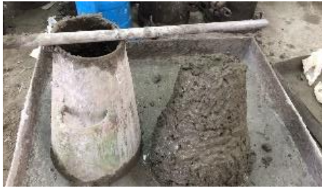
Figure 7. Slump test result for 0.8% CF 615.
