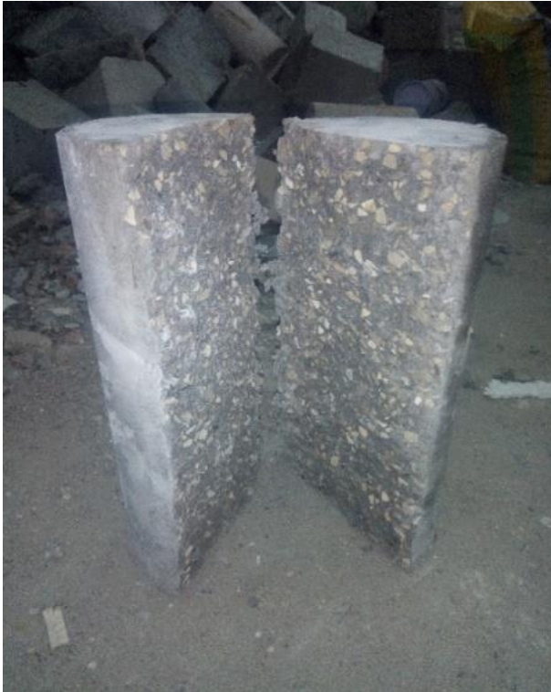
Fig. 3. Sample of Brazilian tensile test.
