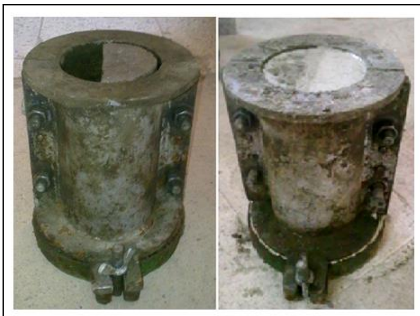
Fig. 3. Composite specimen for splitting tensile strength.
