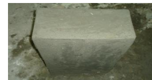
Figure 10: Column specimen after apply plastering works by mortar (SP).
