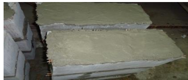
Figure 6: Column specimens after filling the holes by mortar (SP).
