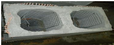
Figure 5: Steel wire mesh box reinforcement arrangement inside the holes of column specimens.
