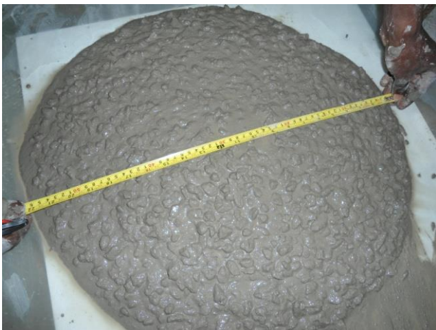
Fig. 1. Slump flow test measurement.
