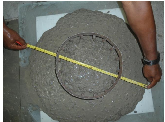
(a) J-ring flow test
