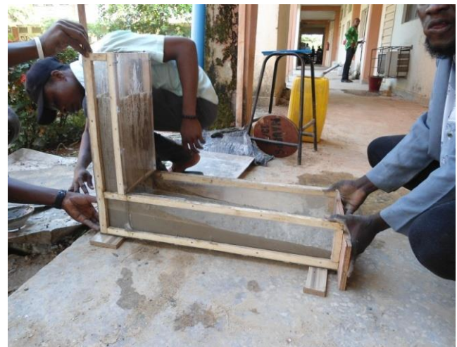
(b) L-box flow test
