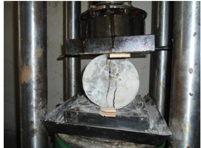
Fig. 7. Splitting tensile testing.
