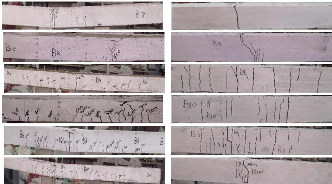
Crack Pattern from side of the beam
