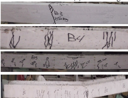
Crack Pattern from side of the beam
