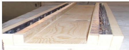
Figure 3. U shape Wooden Mold
