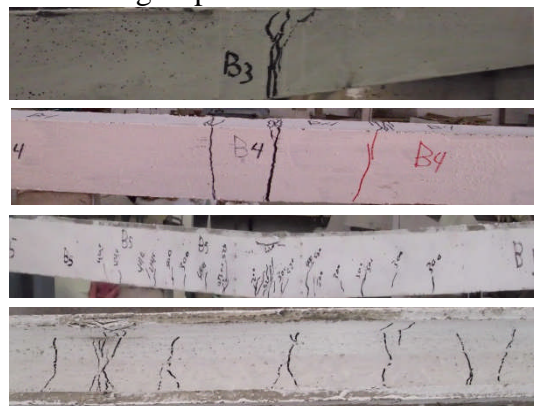
Crack Pattern from bottom of the beam
