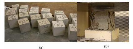
Figure 1 (a, b). Testing compressive strength of concrete specimens: (a) specimens before testing; (b) after testing
