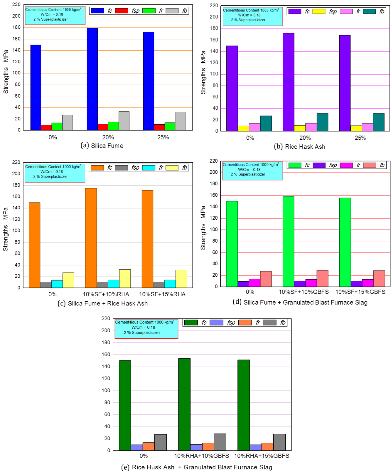
Fig. 7. Effect of replacement materials on different strengths of HSC: (a) Silica Fume; (b) Rice Husk Ash; (c) Silica Fume + Rice Husk Ash; (d) Silica Fume+ Granulated Blast Furnace Slag; (e) Rich Husk Ash +Granulated Blast Furnace Slag.
