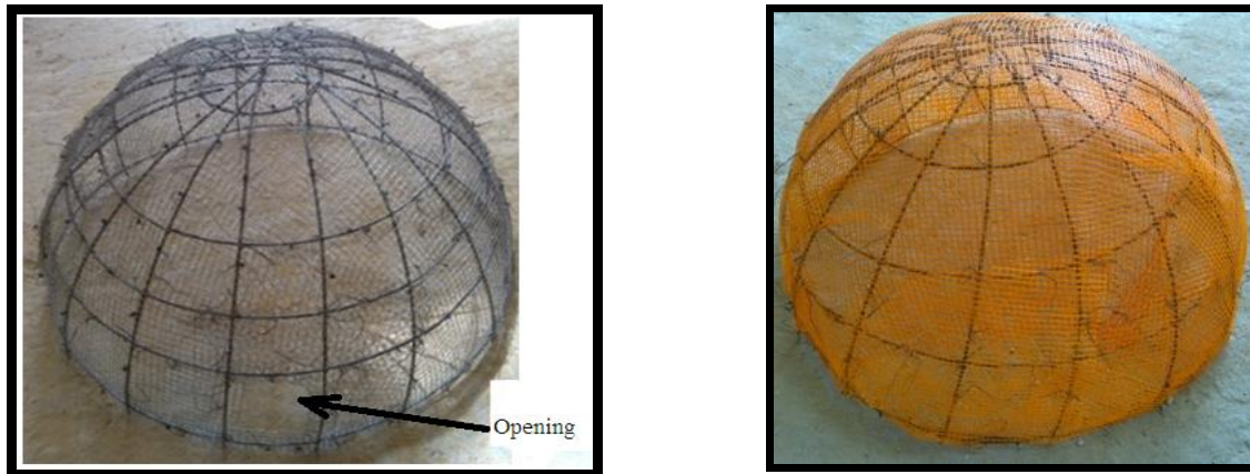
Figure 5. The reinforcements of specimens; a) D2 to the left b) D3 to the right
