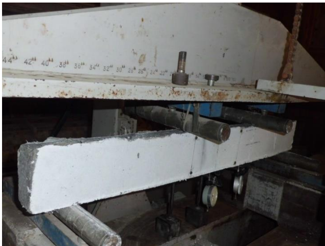
Fig. 18. ELE flexural 100KN testing machine.
