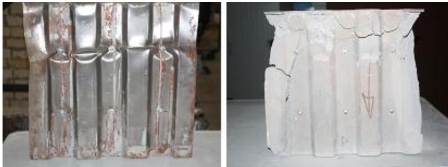
(c) failure mode of specimen with welded edge
