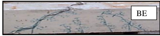
Figure 28. Crack Pattern for beam (BE) after 15 days of Corrosion Acceleration
