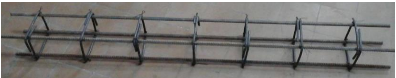
Fig. 2. Upper and lower specimen reinforcement.
