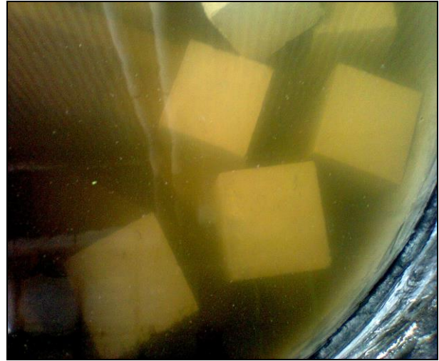
Figure 8: Colour of hydrochloric acid solution after 300 hours of immersion.
