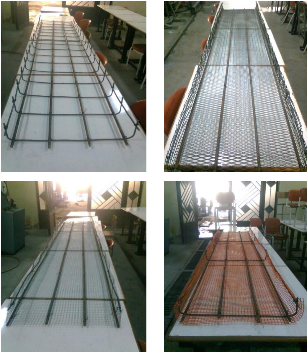
Fig. 3. Reinforcement configuration of U shape slabs.
