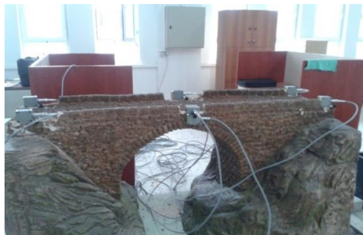
Fig. 2. Test setup of reduced-scaled bridge model.
