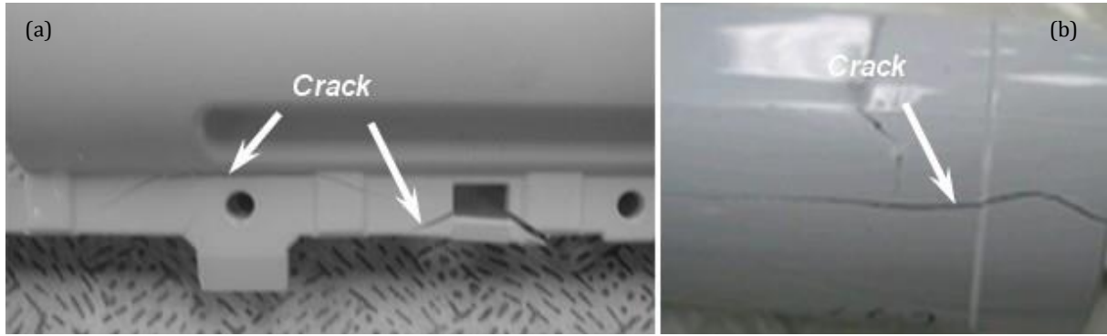
Fig. 7. Failed products in field and crack after 1 st ALT: (a) Failed products in field; (b) crack after 1 st ALT.
