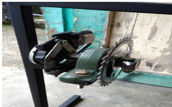
Gambar 4. Motor Power Window , Poros, Bearing Dan Roda Gigi
