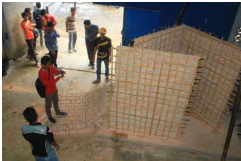
Figure 7. Bamboo wall after shake table testing
