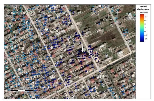
Figure 7. Detailed view of PSI results in one of the areas with maximal negative vertical displacement rates (up to -30 mm/year).
