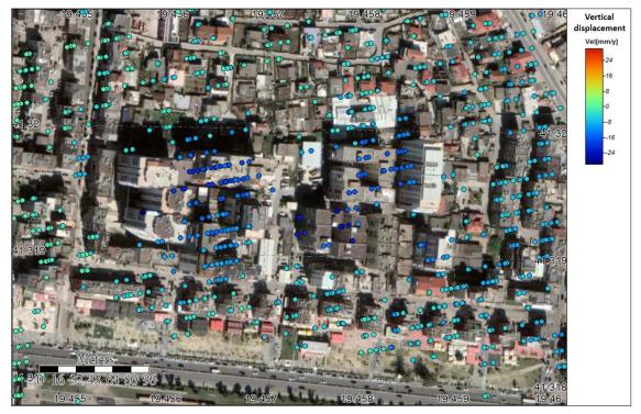
Figure 8. Detailed view of PSI results in one of the areas with maximal negative vertical displacement rates (up to -30 mm/year).
