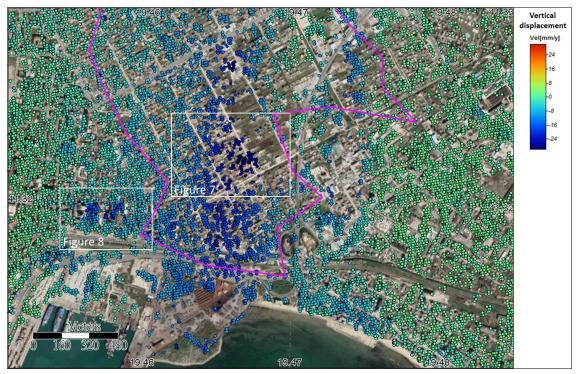
Figure 6. Closer view of the major ground subsidence zones detected by the PSI analysis of the Sentinel-1 SAR images, plotted onto Google Earth<sup>TM</sup> image. The ground displacement rates are shown in mm/year. The contour of the former marsh digitized from the Corona satellite image of Figure 1a is plotted onto the image for reference (magenta color line).
