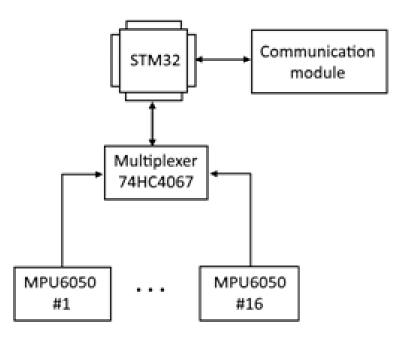
Figure 3. System block diagram
