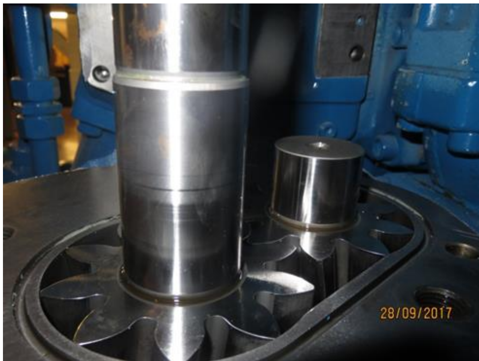
Figure 2.2 pump gears have 10 teeth
