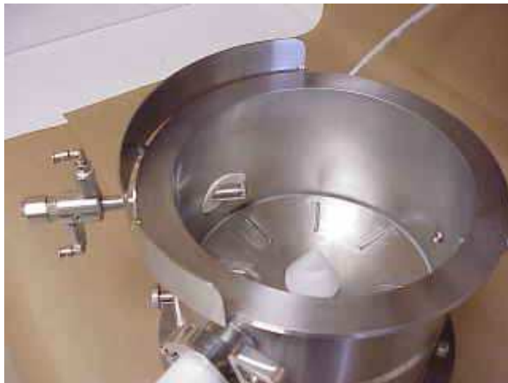
Figure 6: Rotor-disk fluid-bed product container with rotor-disk insert and spray gun (97).
