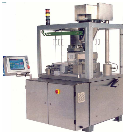
Figure 15: Tamp capsule filling machine with color touch-screen control (left; 226).
