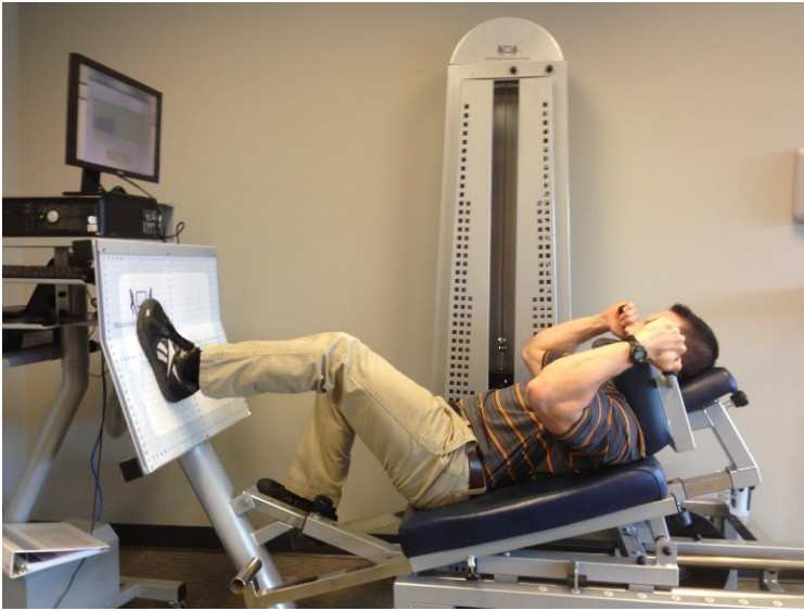
Figure 5. Patient performing a maximal isometric squat test on the Monitored Rehab Systems Computerized Leg Press Machine.
