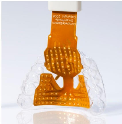
Figure 4. Custom-made SmartPalate® for the Complete Speech Palatometer System. For more information visit:
