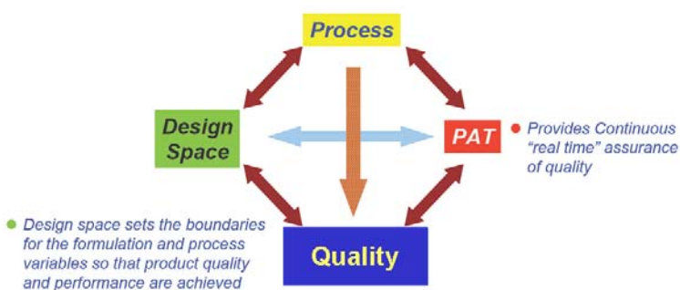
Figure 1.1. The inter-relationship between PAT, design space, and pharmaceutical manufacturing. Adapted from R.C. Lyon, Process monitoring of pilot-scale pharmaceutical blends by near-infrared chemical imaging and spectroscopy, Eastern Analytical Symposium (EAS), Somerset, NJ, 2006.
