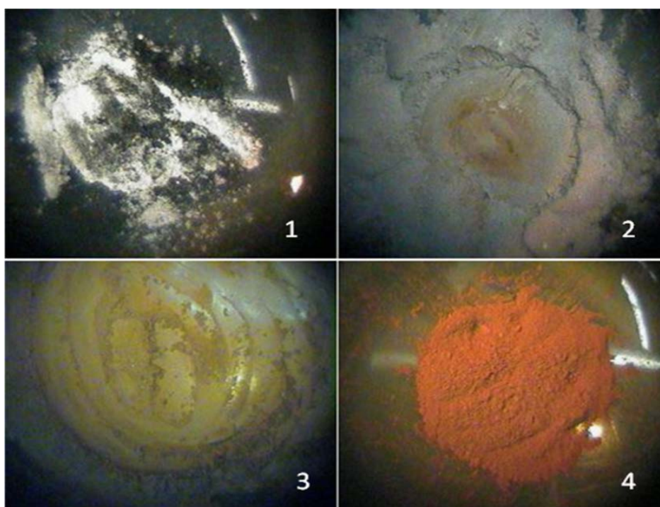
Fig. 5-3: Color change observed upon grinding FeCl 3 with \alpha -Na 3 PO 3 S. The reaction proceeds from 1 to 4 over the course of ~10 minutes of grinding in a mortar with pestle.
