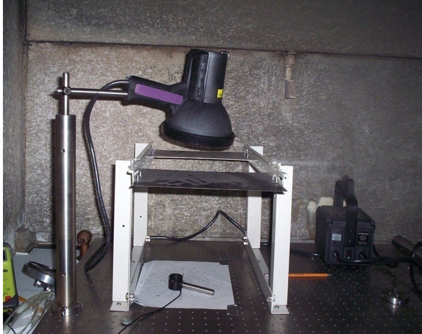
Figure 2.6 Completed direct shutter system with UV lamp and mirror. Setup was still located in a fume hood
