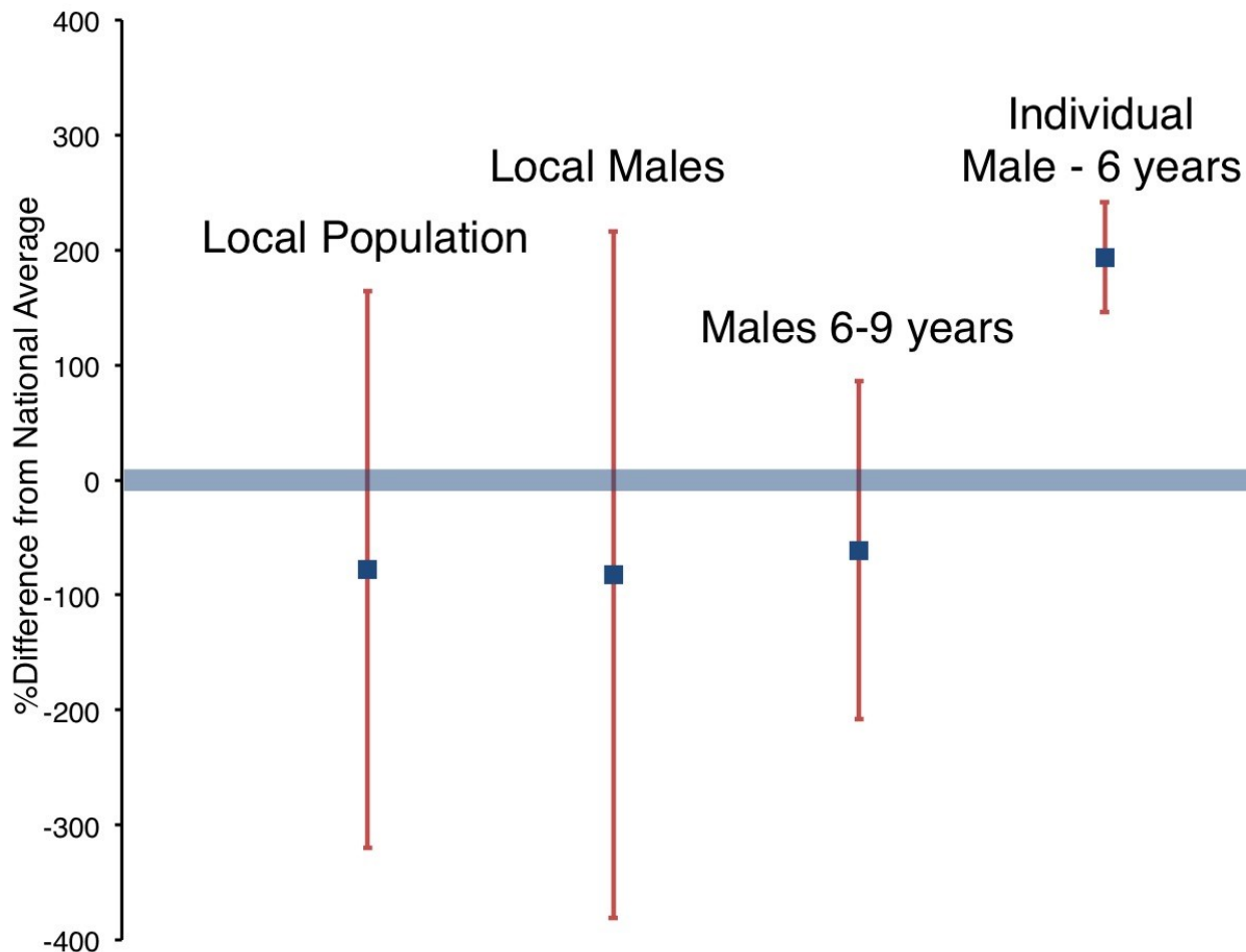
Figure 3.10: Mean difference from national average of metolachlor in regional collaborative study, 95% CI shown (n = 30x5, 27x5, 15x5, 5, respectively). Grey bar represents 95% confidence of national average.
