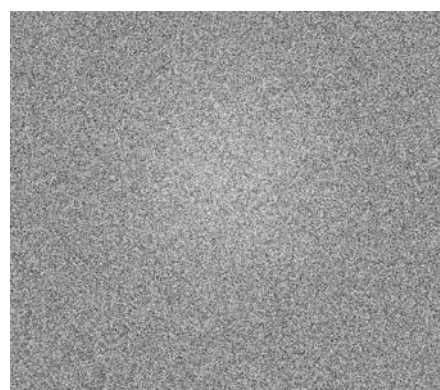
Figure 2: Two dimensional model data generated from a Gaussian and uniform random numbers. Mixing ratio is 1:7. The image is 721×721 pixels and monochrome.
