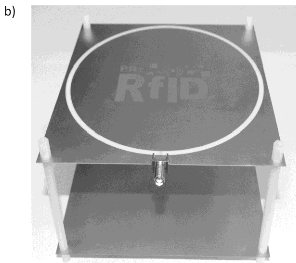
Fig. 3. Constituent antenna of phased array for RWD: a) model, b) practical solution.
